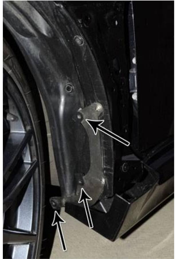
With three DRT screws, three DRT washers and the front DRT mud flap (it's smaller than the rear mud flaps and make sure the DRT logo is facing the rear of the car), with a Phillips screwdriver take screw and washer and line it up to the top hole of the mud flap and top bracket clip. Screw it in a bit (not all the way so you can align the mud flap) and take two screws and two plastic washers and screw in the two remaining clips, but make sure it's not tight so you can adjust it.
