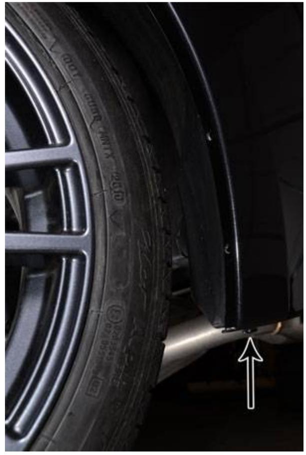
While gently pulling the rear bumper cover take the DRT rear metal bracket and place it between the bumper itself and the plastic cover. Align the bottom tab with the hole of the clip you just removed.
