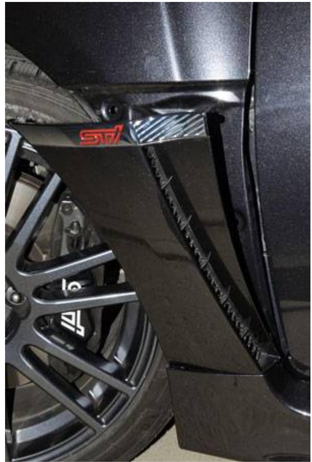
Use a Phillips screwdriver to loosen up the two clips in the fender wall and then use a Flat head screwdriver to carefully remove the two clips.
