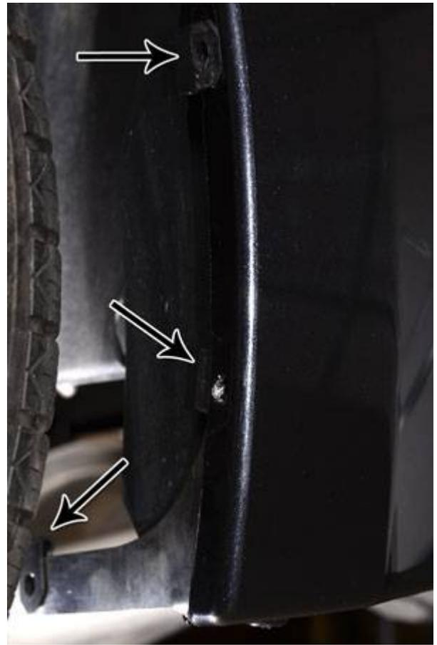
With one screw, a washer and the rear mud flap (it's larger than the front mud flaps and make sure the DRT logo is facing the rear of the car), take the screw and washer and line it up to the top hole of the mud flap and top bracket clip. Screw it in a bit (not all the way so you can align the mud flap) and take two screws and two plastic washers and screw in the two remaining clips, but make sure it's not tight so you can adjust it.
