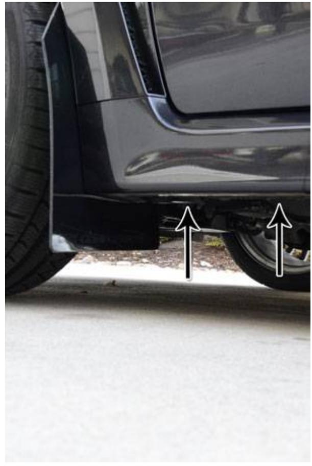
Now gently pull the plastic fender piece from the top and work your way down. The top half is easy to pull off, but note that the bottom is attached by a tab that you have to shift slightly down while removing it.
