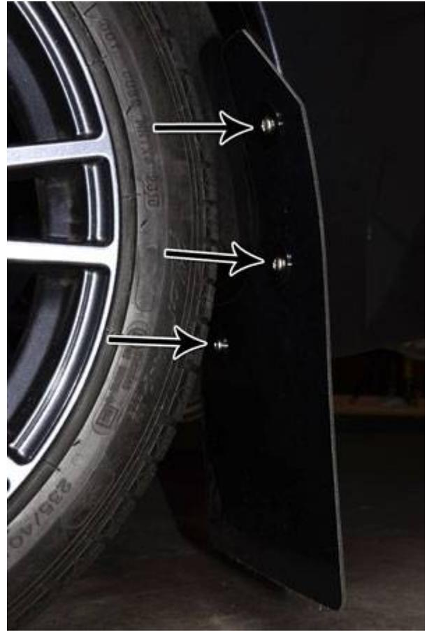
Look at the mud flap and make sure it's aligned to your preference. Then tighten the three screws (without over tightening them).
